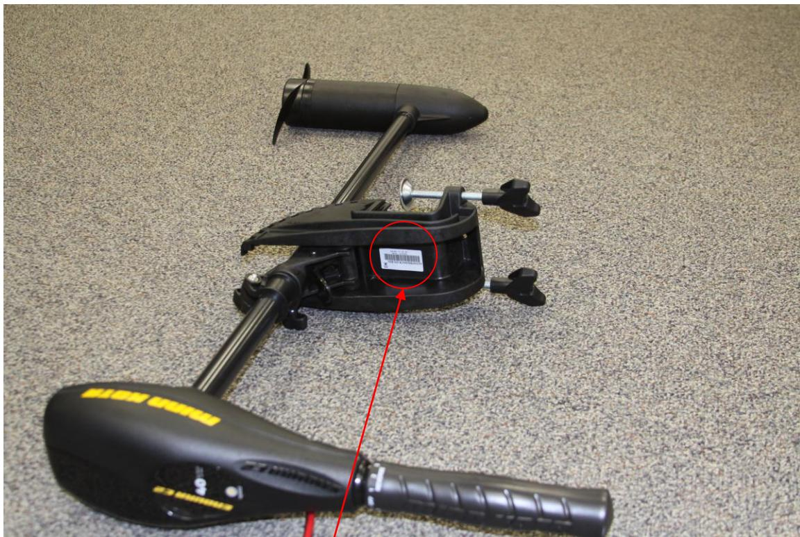
On the Endura models the serial number is located on the top of the mounting bracket.
