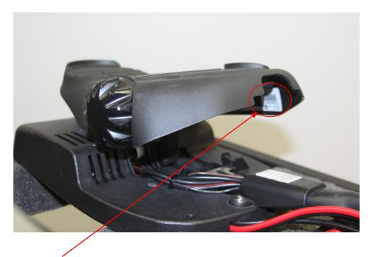
The serial number on Fortrex, Maxxum and Edge foot controlled models is located on the inside edge of the foot pedal under the momentary switch.
