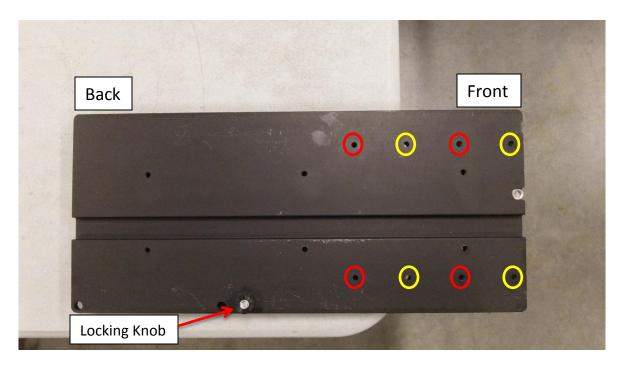
To mount the Terrova/PowerDrive V2 you will need to use *either* the 4 red holes or the 4 yellow holes on the MKA-47 quick release bracket.
