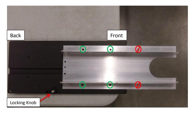
You will *only* use the 4 rear mounting holes (labeled in green) on the Terrova/PowerDrive V2 base. This will ensure that the shaft has proper clearance when the motor is deployed.
