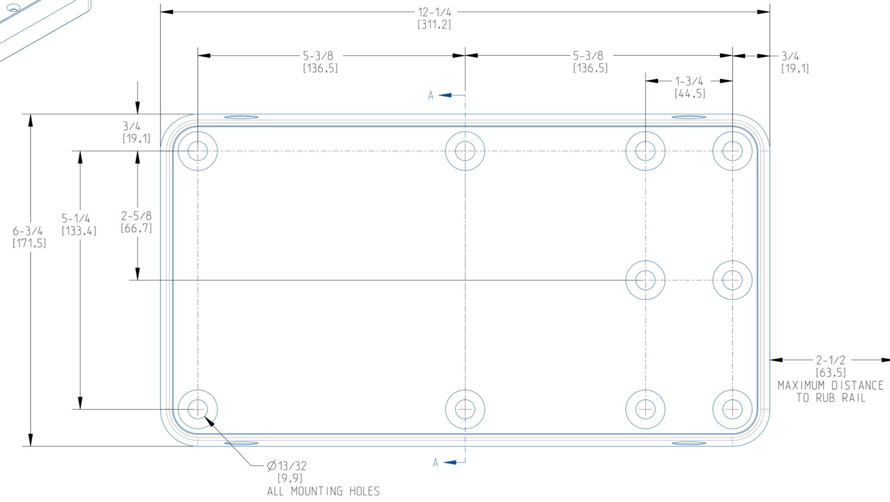
FASTENER HEAD TO BE FLUSH OR RECESSED FROM TOP SURFACE WHEN INSTALLED
