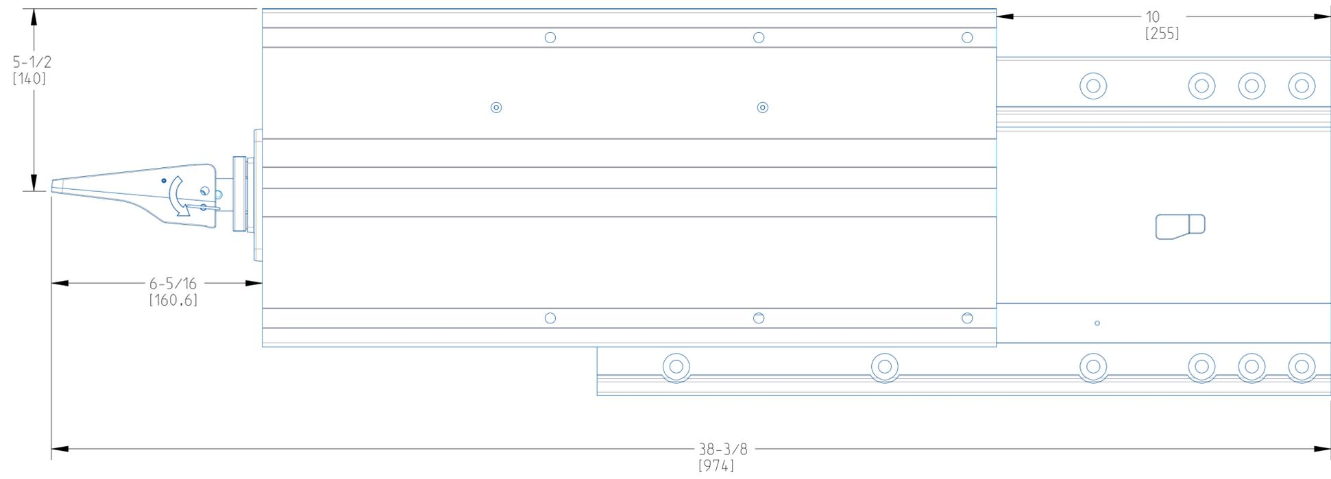
UNLOCKED POSITION WITH HANDLE THROWN STORAGE POSITION TOP PLATE SLID FOR CLEARANCE PURPOSES
