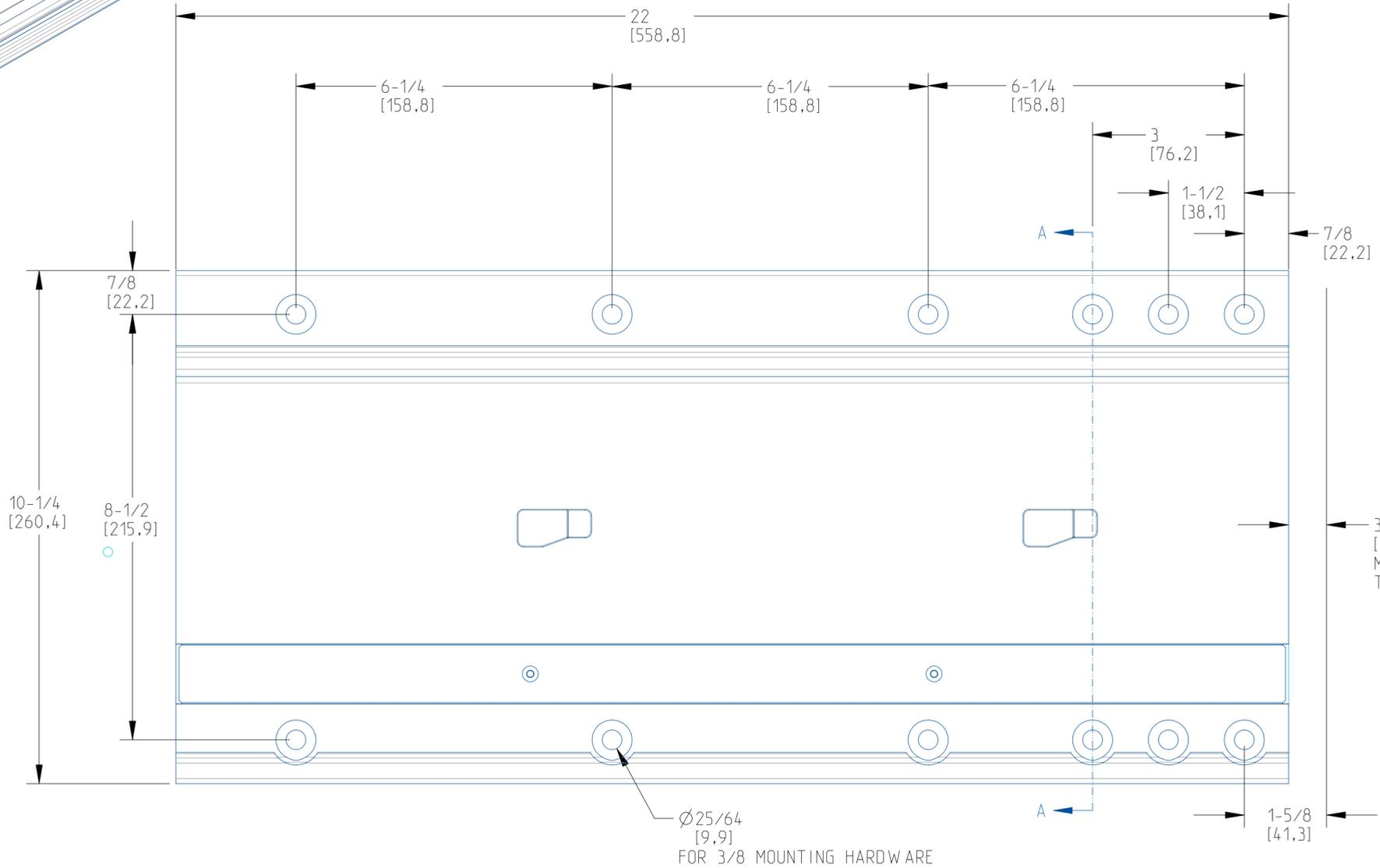
FASTENER HEAD TO BE FLUSH OR RECESSED FROM MOUNTING SURFACE WHEN INSTALLED
