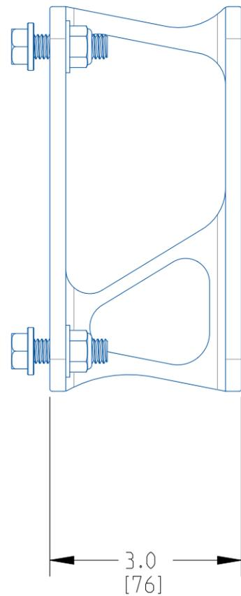
USE 7/16 DRILLBIT WHEN DRILLING HOLES
