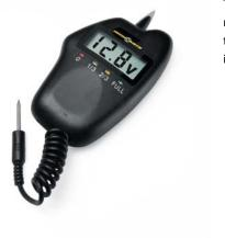
To activate the battery meter touch the probe at the end of the coil cord to the negative post of a battery and touch the probe built into the body of the meter to the positive post of the same battery (as shown below). If the battery voltage is a minimum of 5 volts the meter will turn on.
