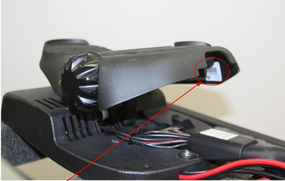
The serial number on Fortrex, Maxxum and Edge foot controlled models is located on the inside edge of the foot pedal under the momentary switch.
