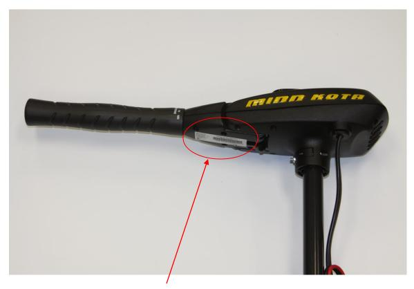
On the Traxxis models the serial number is located on the under side of the pivot handle.
