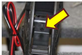
Figure 15: Below view of bracket, hole for T-Bar indicated by arrow
