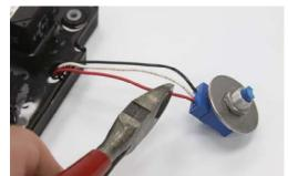
2. Insert the matching colored wires into the connectors and pinch them closed with pliers.
