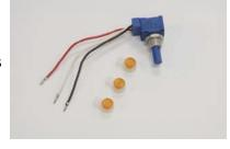
1. Cut the three (3) wires connected to the faulty/damaged potentiometer and clip the pin terminals from the ends of the wires attached to the replacement potentiometer.
