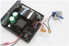
3. Complete the repair by installing the new potentiometer in the control box and re-install the cover and screws.
